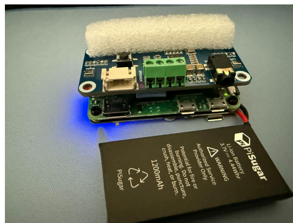
Figure 3.2.4 Testing of the WM8960 HAT
